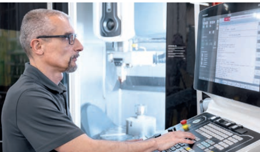
Alternating between laser deposition welding and milling enables the production of highly complex components and the repair of defective workpieces.
