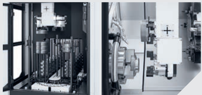
1. Stacking magazine 35 kg load capacity per pallet position 2. Double gripper with 2x5 kg load capacity
