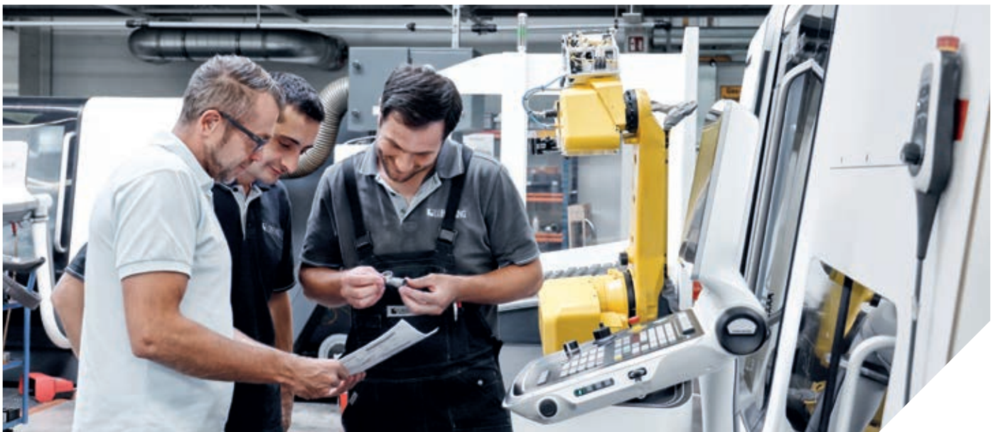
LÜBBERING supports its skilled staff on the CTC turn & mill centres with a Robo2Go from DMG MORI.
