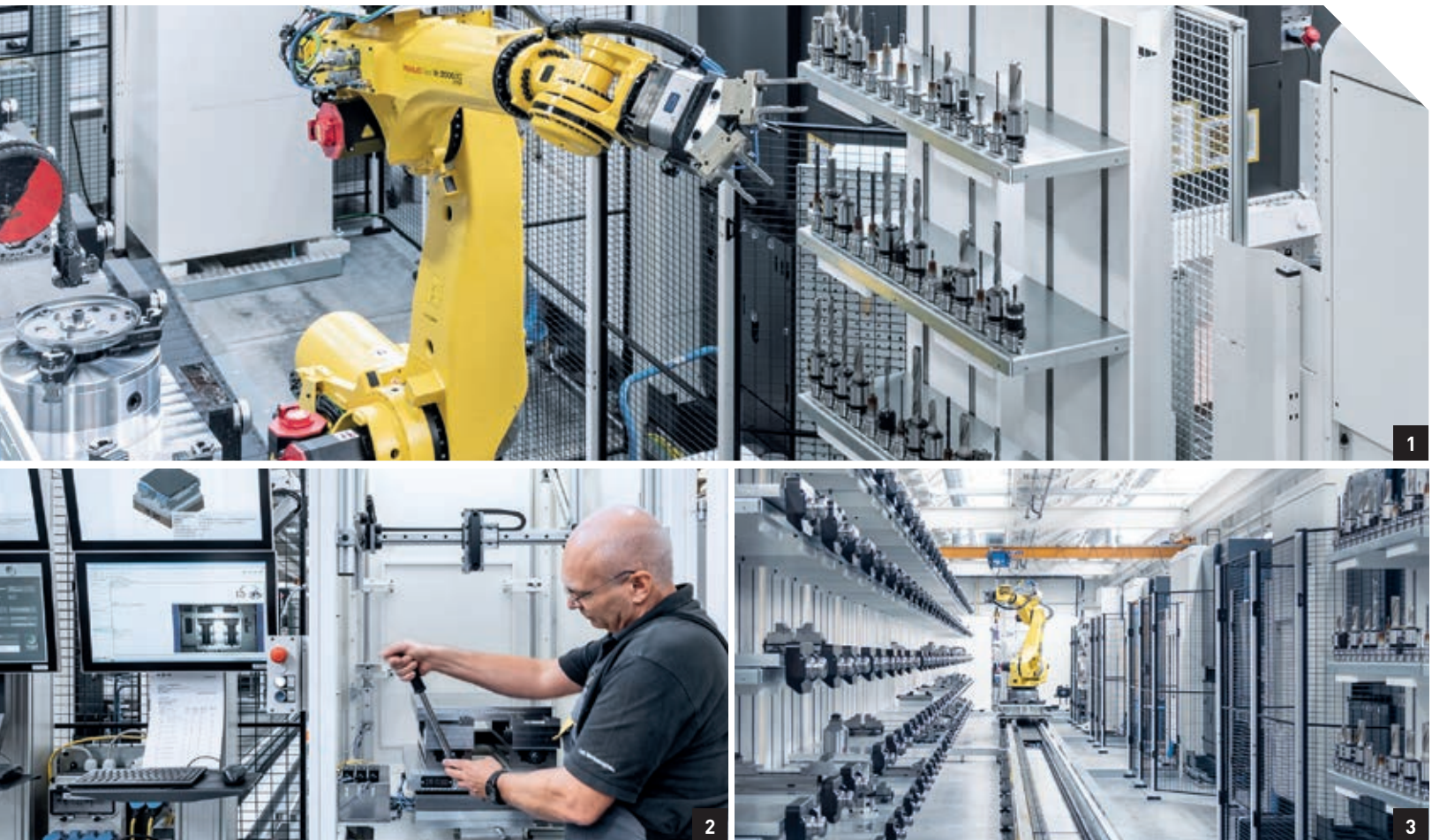
1. In addition to the 120 tool stations per machine, the automation also includes 105 stations for special tools. 2. The set-up stations are equipped with a camera system developed by Schaeffler, which enables the operator to set a zero point on the PC. 3. The 30-metre-long system includes five DMU 80 eVo linear machines, a tool presetter including a set-up station for tools, two set-up stations for workpieces and an off-load station.
