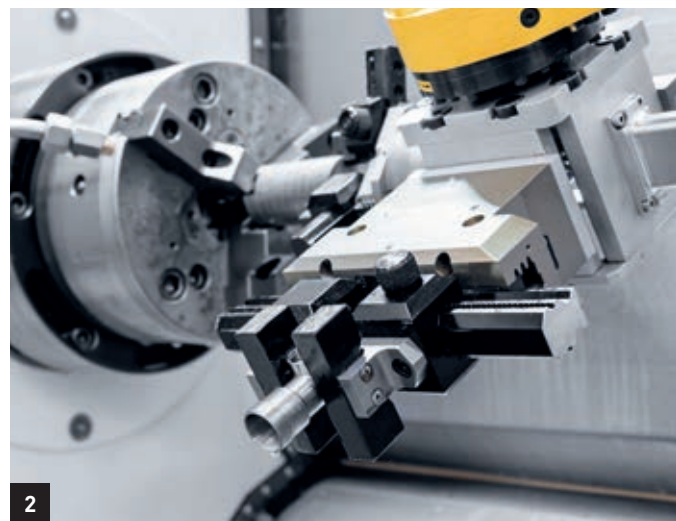
1. The magazine of the Robo2Go has space for 72 workpieces. 2. The Robo2Go unloads the finished parts from the counter-spindle and loads the main spindle with new blanks – fully automatically.
