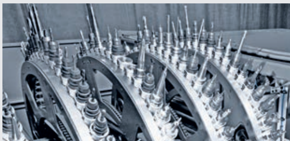
Outer wheel with 63 available tool pockets, Inner wheels with 60 available tool pockets.
