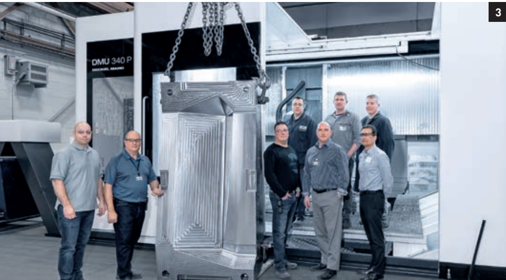
1. Sophisticated 5-axis machining on the DMC 85 monoBLOCK 2. With its three-pallet system, the DMC 85 monoBLOCK allows up to 20 hours of unattended operation 3. The DMU 340 P machines large workpieces to an accuracy of \pm 0.05 mm
