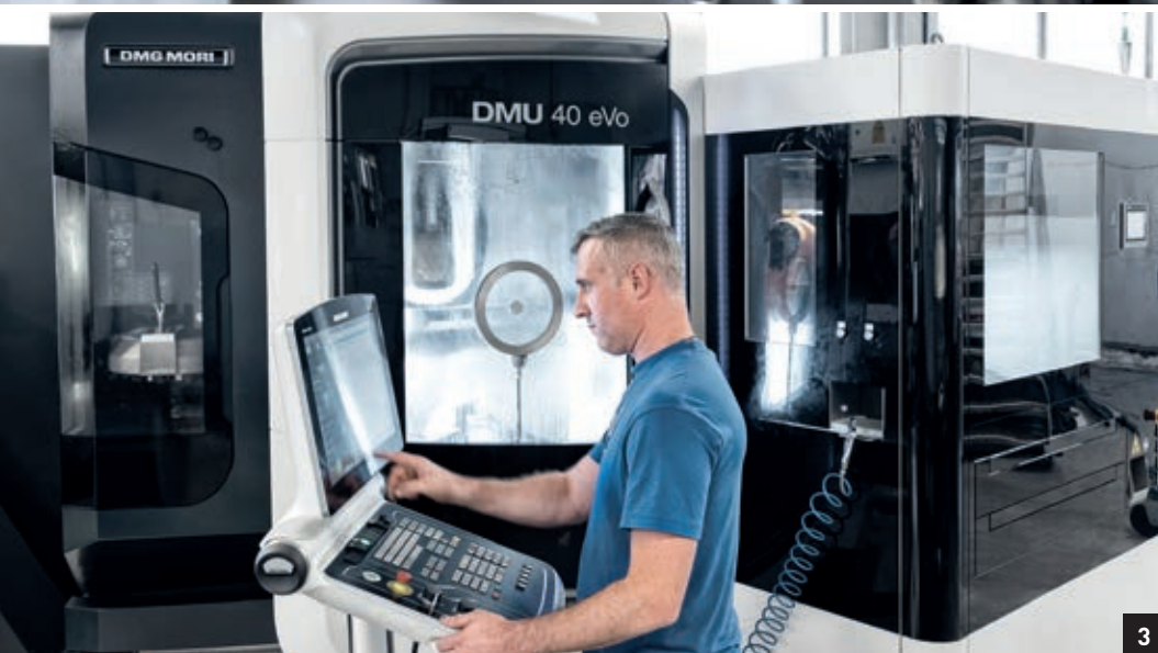
1. The DMG MORI production cell was developed as a dedicated turnkey project for vane machining 2. Accurate results to a tolerance of less than one hundredth of a millimetre in 3-shift operation 3. Perfect accessibility, also for manual operation
