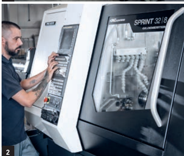
1. O.M.Z. currently operates 28 automatic turning centres from DMG MORI 2. The SPRINT 32|8 has a footprint of just 2.8 m 2 3. O.M.Z. boosts productivity with bar feeders
