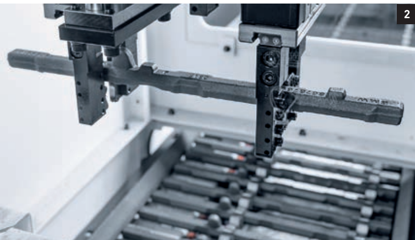
1. In 2016, Eisenwerk Erla established an automated machine shop comprising a total of 18 linked NLX 2500s 2. The robot removes the blanks from the conveyor belt
