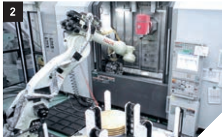
1. Example of a workpiece with a blank weight between 40 and 50 kg 2. Automatic robotic loading of the NT 4300 DCG
