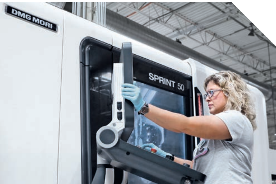
Operator Erica Williams working on the SPRINT 50. The production turning machine enables automatic bar machining and turning of chuck parts with up to 36 tool stations.
